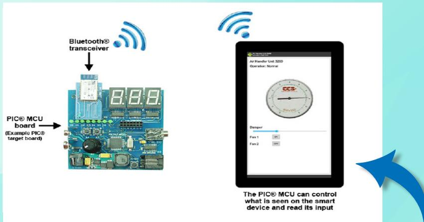
Use the EZApp library to quickly create a wireless sensor or controller on a PIC<sup>®</sup> MCU that may be viewed and displayed on a mobile device using Bluetooth<sup>®</sup> included in CCS IDE Compilers. Drivers, examples and development boards for the Microchip RN-4020 Bluetooth<sup>®</sup> module.
