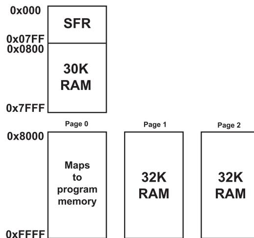
From C, the compiler will allocate variables into the first page of extended RAM only. To access additional memory special functions must be used.
