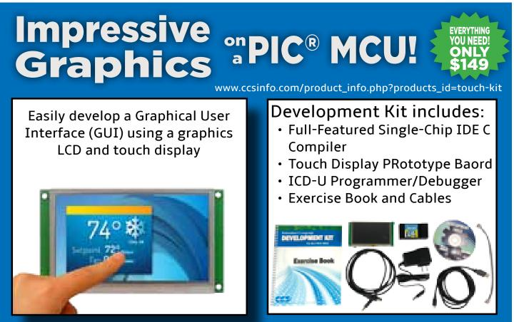
The new Touch Display 4.3 Development Kit is all that is needed to develop a GUI using the Graphics and Touch Library. Powered by a PIC24EP512GU810 it has a 4.3" 480x272 TFT display with a resistive touch-screen, a 256 megabyte flash, capable of storing hundreds of 480x272 images and custom fonts, a USB connection and 8 digital I/O pins that can be used for external inputs and outputs. No device programmer required - includes onboard programming capabilites.
